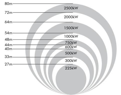
*Fig 2: The industry standard continues to ignore the fact that the total blade surface area is a critical factor in relationship to the total rotor swept area; that is, if the blade surface area is 10% of the rotor swept area, then 90% of the total cubic airflow and available kinetic energy passing through the rotor disc area is not contributing to energy transfer.*
